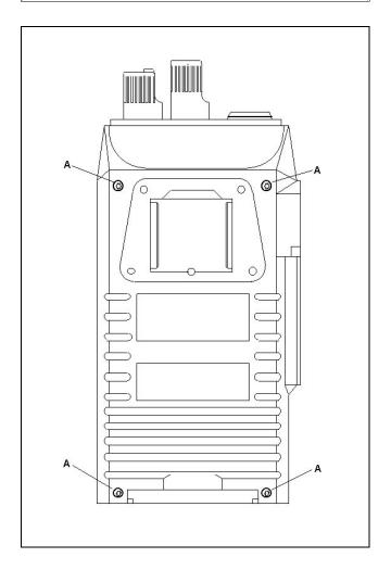
Figure 6 - Front And Rear Cover Separation
